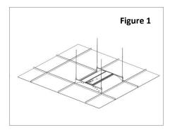
1. Install the luminaire into the reserved space in the ceiling. Attach the luminaire by the steel hook/safety cable.
