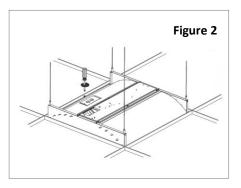
2. Remove electrical enclosure cover, and remove knockout for AC line input wires.
