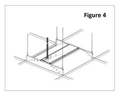
4. Push all lead wires into the electrical enclosure. Reattach electrical enclosure cover; make sure no wires are pinched.
